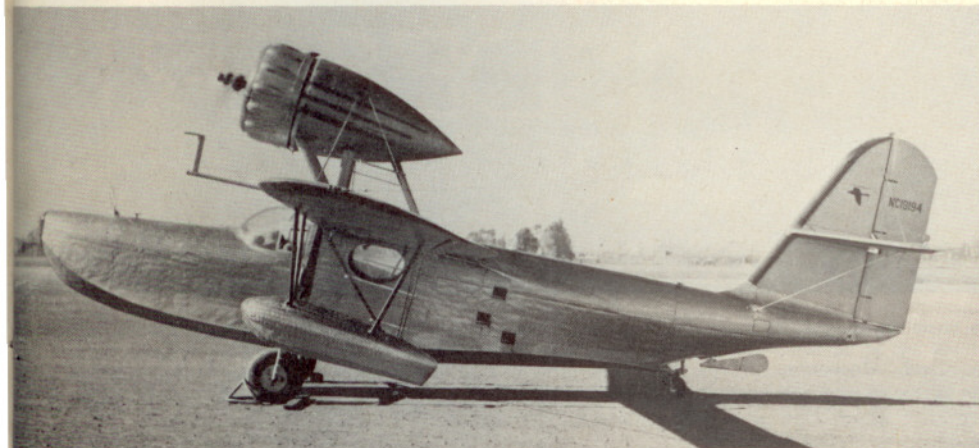
Fleetwings F-505, the last Sea Bird built. Note extreme upward angle of engine thrust line and negative angle of incidence of horizontal tail to reduce nose-over effect of high-mounted engine. Compare one-piece bubble canopy of F-5 to flat-panel built-up type of original F-4 and note larger side windows on F-5. E. M. Sommerich photo
